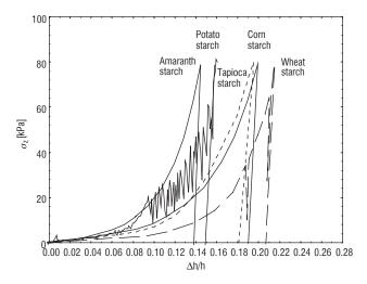
FIGURE 9. Stress strain relationships in uniaxial compression of examined starches.
