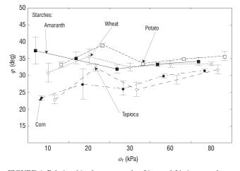
FIGURE 6. Relationships between angle of internal friction  $\varphi$  and consolidation reference stress  $\sigma_r$  for the tested starches.
