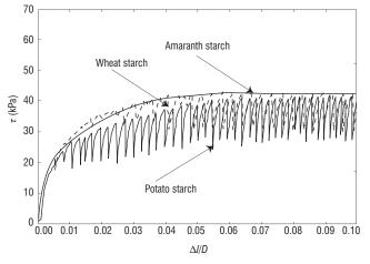
FIGURE 5. Shear stress  $\tau$  – relative displacement  $\Delta l/D$  relationship of potato, wheat and amaranth starch for normal pressure  $\sigma$  of 60 kPa.
