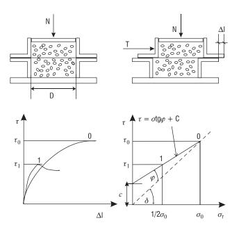
FIGURE 1. Direct shear apparatus and interpretation of experimental data following Eurocode 1:  $\tau$  – shear stress [kPa],  $\sigma_r$  – consolidation reference stress [kPa],  $\Delta l$  – relative displacement.
