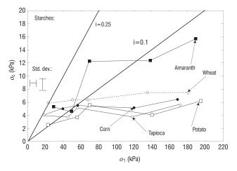
FIGURE 8. Flow functions  $FF = \sigma_c(\sigma_l)$  of tested starches.
