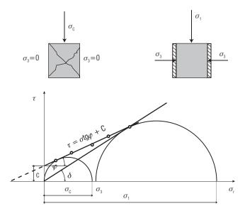
FIGURE 2. Determination of flow function  $FF = \sigma_c(\sigma_1)$  of powder.
