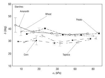
FIGURE 7. Relationships between effective angle of internal friction  $\delta$  and consolidation reference stress  $\sigma_r$  for the tested starches.
